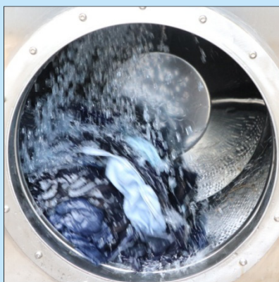
專利撥水式內膽，無泵水循環，實現超低水比染色，節約用水及染料 Patented bail type inner drum and pump-free water circulation enable extra low liquor ratio, with minimal water and dye consumption
