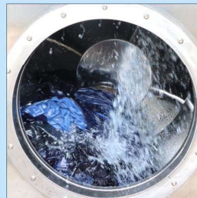
專利撥水式內膽，無泵水循環，實現超低水比染色，節約用水及染料 Patented bail type inner drum and pump-free water circulation enable extra low liquor ratio, with minimal water and dye consumption
