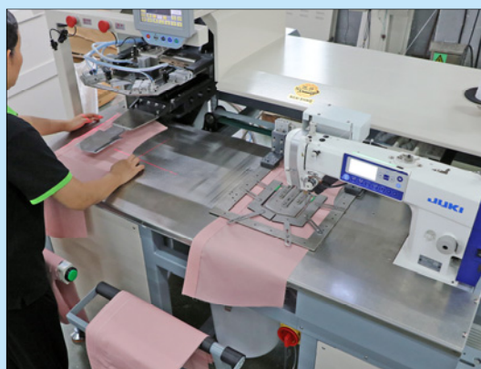
3.機器自動貼袋車縫及收料 Automatic pocket setting and collecting
