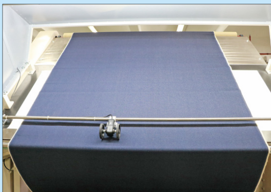
驗布操作 Fabric inspecting operation
