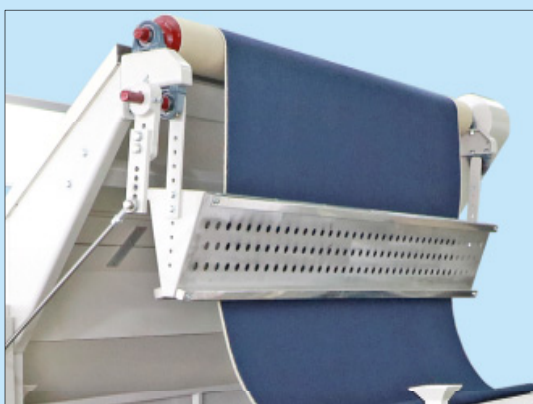
鬆布操作 Fabric loosening operation
