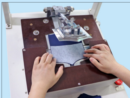
將袋布放在發熱板上 Place material on heating platform
