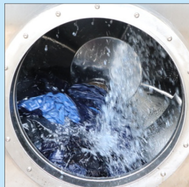
專利撥水式內膽，無泵水循環，實現超低水比染色，節約用水及染料 Patented bail type inner drum and pump-free water circulation enable ultra low liquor ratio, with minimal consumption of water and dyes
