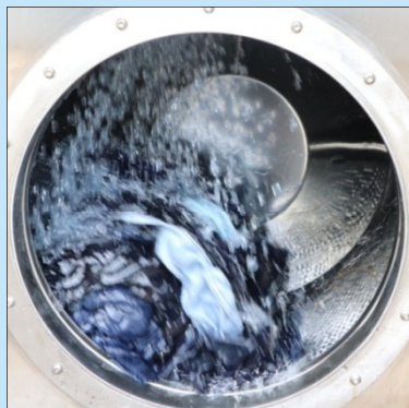
專利撥水式內膽，無泵水循環，實現超低水比染色，節約用水及染料 Patented bail type inner drum and pump-free water circulation enable ultra low liquor ratio, with minimal consumption of water and dyes
