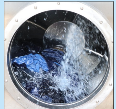
專利撥水式內膽，無泵水循環，實現超低水比染色，節約用水及染料 Patented bail type inner drum and pump-free water circulation enable ultra low liquor ratio dyeing process, with minimal consumption of water and dyes
