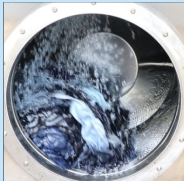
專利撥水式內膽，無泵水循環，實現超低水比染色，節約用水及染料 Patented bail type inner drum and pump-free water circulation enable ultra low liquor ratio dyeing process, with minimal consumption of water and dyes
