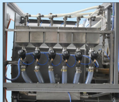
O-I-21-01-05-05 自動入藥水連水泵總成(5L+5L) Automatic Chemical Feeding with Pump Assembly (5L+5L)
