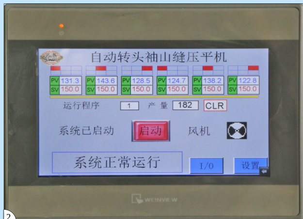
PLC可編程控制器控制及人性化操作界面觸摸顯示屏 操作 Adopt PLC and user friendly touch screen for operation
