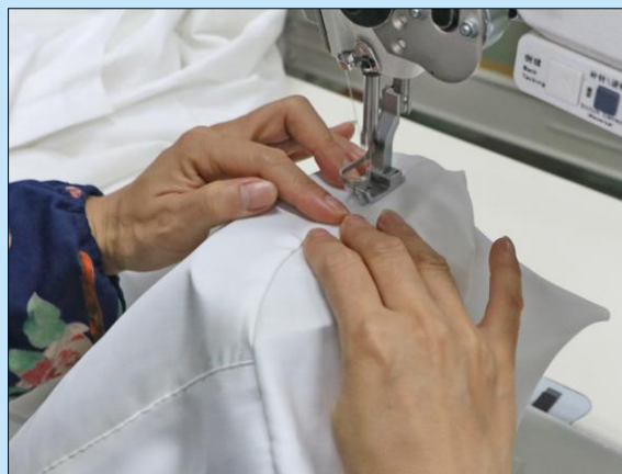
袖圈間線操作 Armhole topstitch operation
