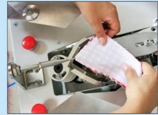
切領咀、反領操作 Collar tip trimming and turning
