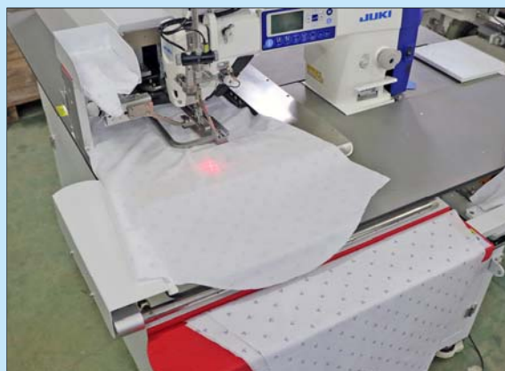
自動袖衩縫紉及自動收料 Automatic sleeve placket sewing & collecting
