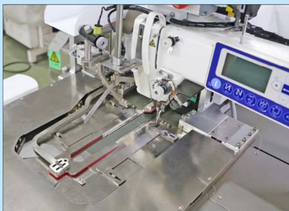
袖衩折疊及輔助壓板裝置 Sleeve placket folding & auxiliary pressing plate device
