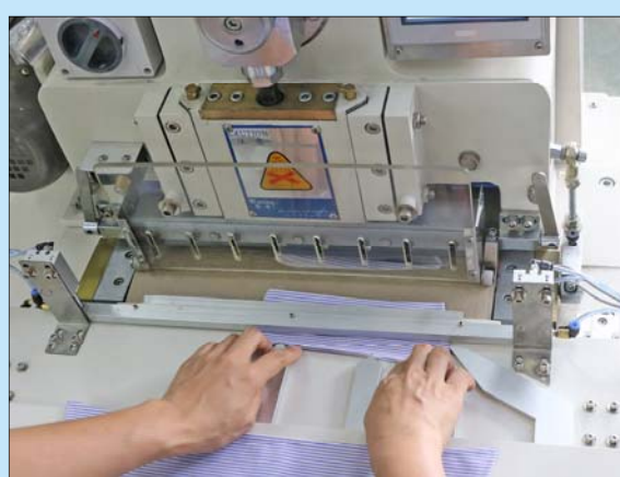
自動送料修領腳操作 Collar trimming operation with automatic feeding
