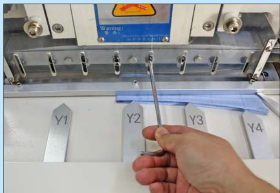
修領腳刀角度調節 Cutting blade angle adjustment
