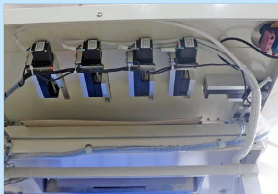
數碼調節XY軸傍位 Digital adjustment of axis XY guide device
