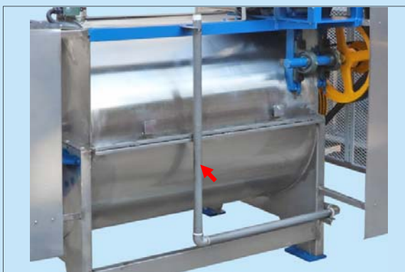
蒸汽直接加溫裝置(NS-2700-70~100) Direct steam heating device (NS-2700-70~100)
