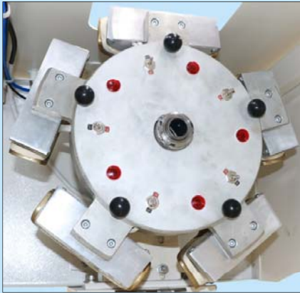
5個不同壓模，滿足不同尺寸需求 5 different-sized moulds cater for different sized collars
