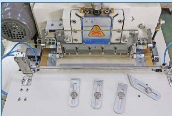
活動傍位及安全罩 Adjustable guide and safety cover
