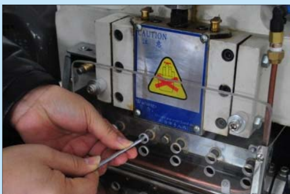
切刀彎度可調校 Could adjust the curve of cutting blade
