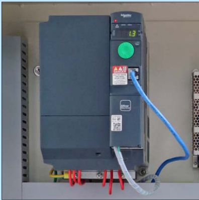
變頻調速控制內膽轉速 Inverter controlled inner drum speed
