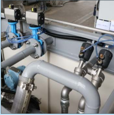
氣動入水/入蒸汽 Pneumatic water/steam feeding
