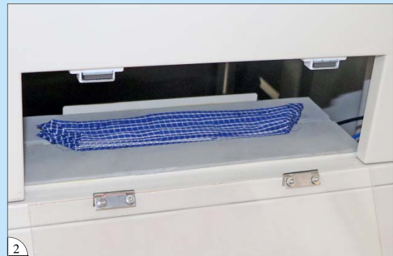
2 自動收料於操作者前方，取料便捷 Automatic stacking in front of the operator, easy to collect the sleeve plackets
