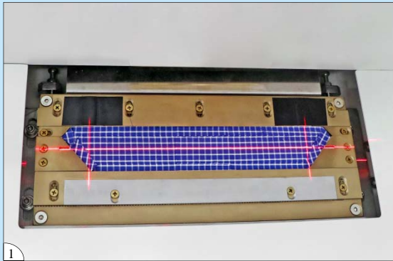
1 下模抽風便於將裁片折邊、貼合完好 Vacuuming of lower mould facilitates folding and flattening fabric piece
