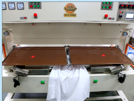
壓布框下壓 Fabric holder closing
