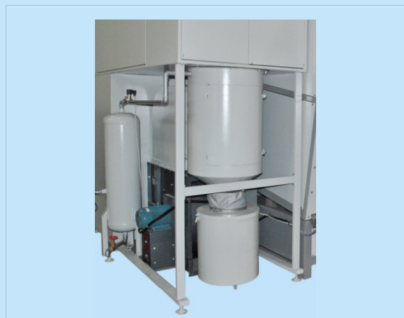
自動除塵箱 Automatic dust collecting device
